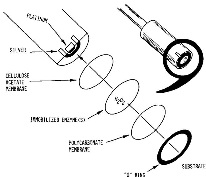
Fig. 1. Model 27 electrode/membrane-immobilized enzyme assembly.
