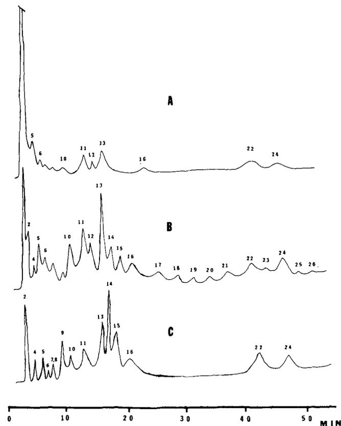
**Fig. 1.** High performance liquid chromatography (Microbondapak C<sub>18</sub>) of fresh beer haze (A, Haze 2; B, Preparation 6) and a cocktail of 16 reference phenolics (C). Gradient: 10–40% solvent B and solvent A. Detection at 280 nm. Peak numbers given in Table I.
