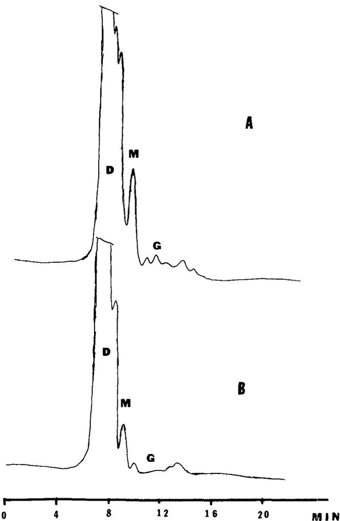
Fig. 6. High performance liquid chromatography (Aminex HPX-87) of forced beer haze (A, Haze 4; B, Haze 4 Sep-pak treated). Detection: differential refractometer. D = dextrin, alcohol-precipitated; M = maltose; G = glucose; F = fructose.
