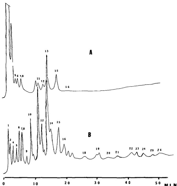
Fig. 2. High performance liquid chromatography (Microbondapak  $C_{18}$ ) of forced beer haze (A, Haze 4; B, Preparation 8). Gradient: 10–40% solvent B in solvent A. Detection at 280 nm. Peak numbers given in Table I.
