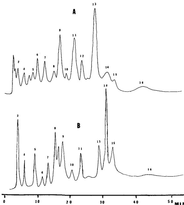
Fig. 4. High performance liquid chromatography (Microbondapak C<sub>18</sub>) of Preparation 8 (A) and a cocktail of 16 reference phenolics (B). Gradient: 10-25% solvent B in solvent A. Detection at 280 nm. Peak numbers given in Table I.
