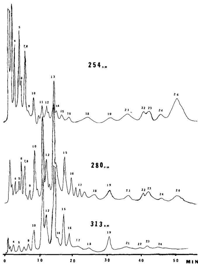
Fig. 3. High performance liquid chromatography (Microbondapak  $C_{18}$ ) of Preparation 8. Gradient: 10–40% solvent B in solvent A. Detection at 254, 280, and 313 nm. Peak numbers given in Table I.
