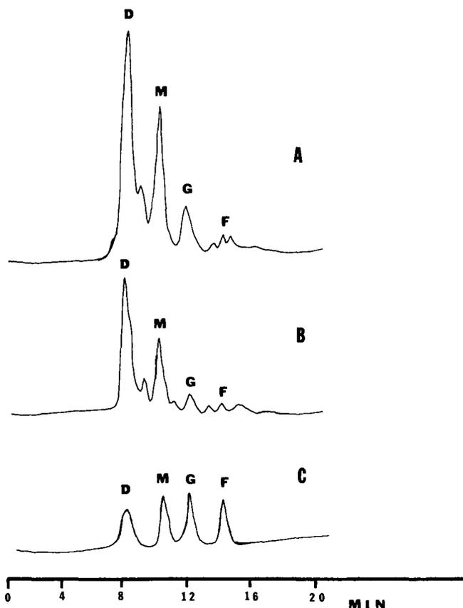
Fig. 5. High performance liquid chromatography (Aminex HPX-87) of fresh beer haze (A, Haze 2; B, Haze 2 Sep-pak treated) and a cocktail of four reference carbohydrates (C). Detection: differential refractomonitor. D = dextrin, alcohol-precipitated; M = maltose; G = glucose; F = fructose.
