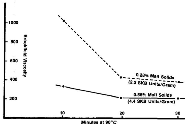
Fig. 7. Liquefaction of 40% jet cooker starch at 90°C by malt infusion (pH 6.5; 0.04% Ca<sup>++</sup> in starch).
