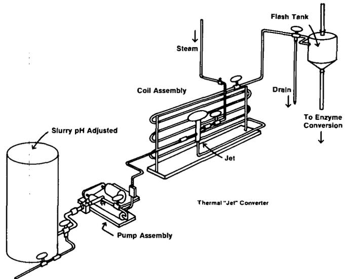
Fig. 6. A jet-cooking process for substrate conversion.
