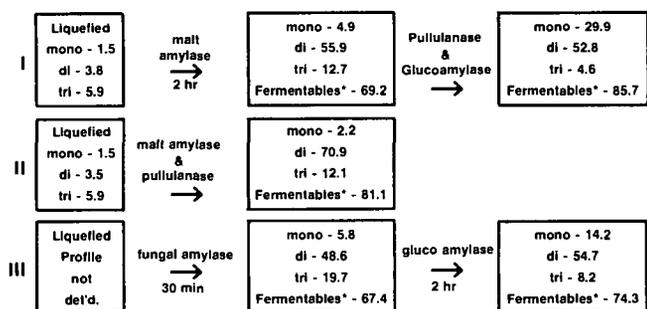
Fig. 8. Conversion of enzyme-liquified starch with 30% dry solids (pH 5.0, 62°C). Syrup profiles expressed as percent carbohydrate. Fermentables - estimated = mono + di + 0.66 tri.
