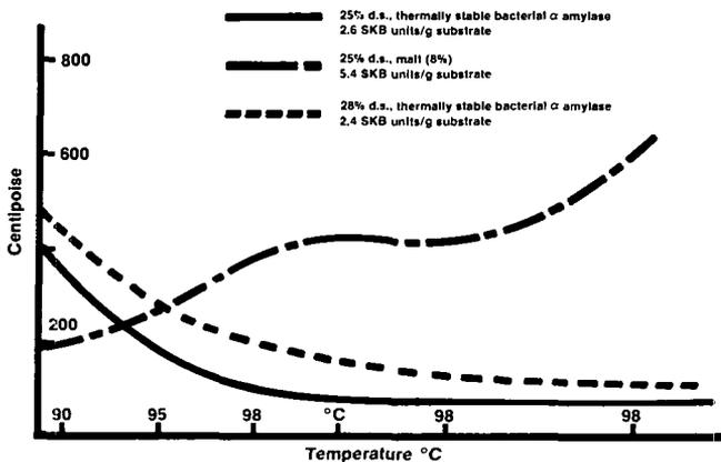
Fig. 5. Viscosity characteristics of batch-converted corn grits. Malt vs thermally stable bacterial  $\alpha$ -amylase. — = 25% d.s., thermally stable bacterial  $\alpha$ -amylase giving 2.6 SKB units per gram of substrate. — — — = 25% d.s., malt (8%) giving 5.4 SKB units per gram of substrate. - - - - = 28% d.s., thermally stable bacterial  $\alpha$ -amylase giving 2.4 SKB units per gram of substrate.
