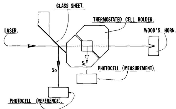
Fig. 1. Schematic diagram of equipment for measurement of chill haze.  $S_0$  = exciting luminous flux,  $S_1$  = scattered flux.
