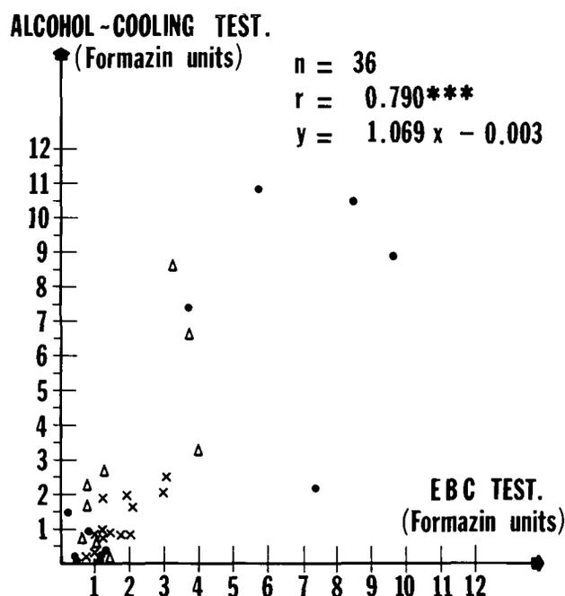
Fig. 4. Correlation between EBC test (14) and alcohol-cooling test (25).  $\Delta$  = Beer from marketplace,  $\bullet$  = pilot plant beer,  $\times$  = beer freshly packaged in the brewery.
