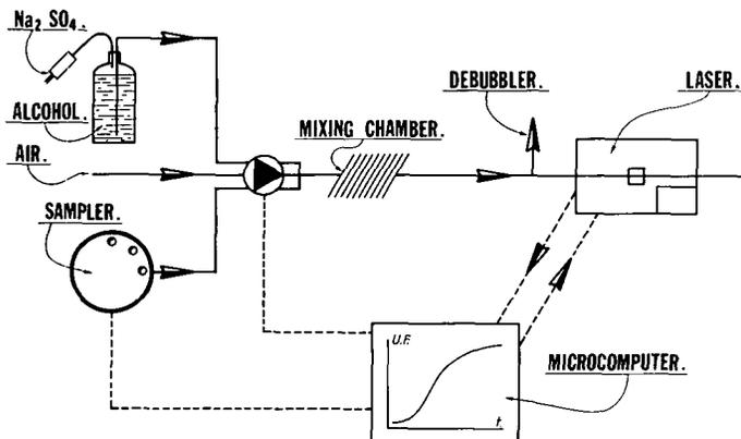
Fig. 2. Layout of equipment for preparing, introducing, and measuring chill haze.
