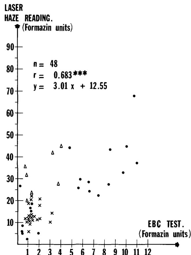
Fig. 3. Correlation between EBC haze liability test (14) and new laser technique.  $\Delta$  = Beer from marketplace,  $\bullet$  = pilot plant beer,  $\times$  = beer freshly packaged in the brewery.
