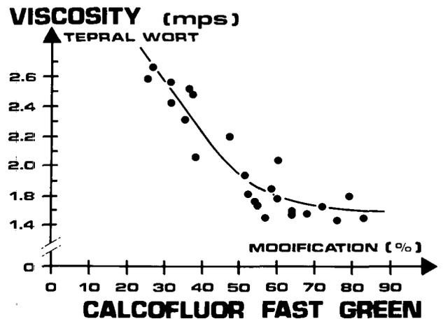
Fig. 3. Relationship between the viscosity of the wort from the TEPRAL mash and percentage modification.
