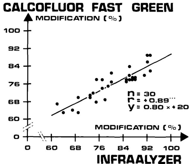
Fig. 5. Test for modification: comparison between results obtained with the InfraAlyzer and by staining of the malt grains.
