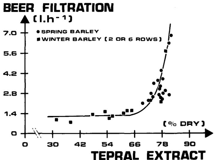
Fig. 6. Relationship between the rate of filtration of beer and the extract yield (TEPRAL mash) from the malt used to make the beer.
