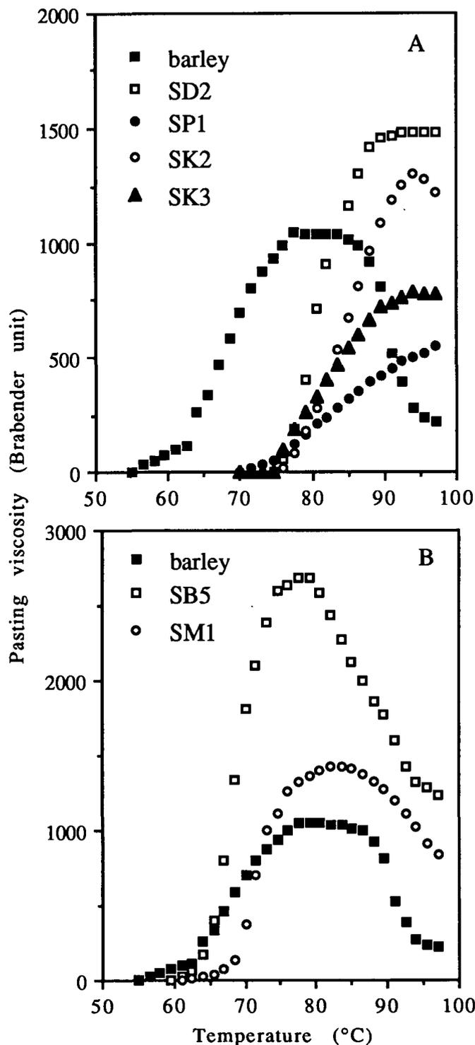
Fig. 2. Brabender viscosity curves for barley and sorghums SD2, SP1, SK2, and SK3 (A) and SB5 and SM1 (B).
