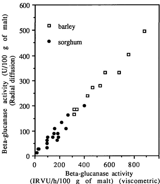
Fig. 5. Comparison of radial diffusion technique and viscometric method for  $\beta$ -glucanase activity in barley and sorghum malts. IRVU = increase in reciprocal viscosity unit.
