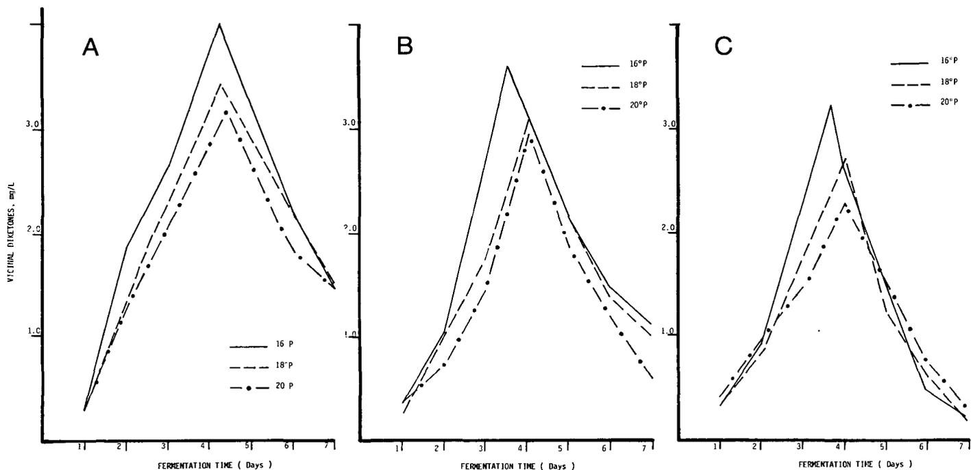
Fig. 6. Vicinal diketone profiles in fermentations of high-gravity worts by *Saccharomyces uvarum* J-3015 at maximum temperatures of A, 16°C; B, 18°C; C, 20°C.
