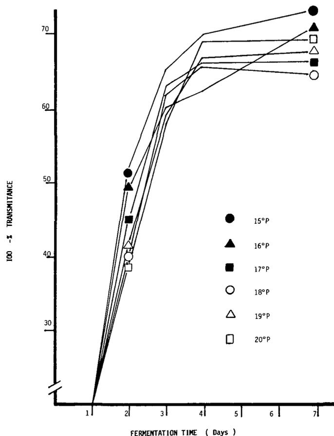
Fig. 2. Effect of carbohydrate concentration on growth of *Saccharomyces uvarum* J-3015.
