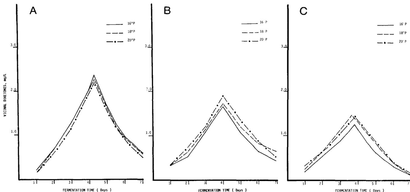
Fig. 7. Vicinal diketone profiles in fermentations of high-gravity worts by *Saccharomyces uvarum* J-2036 at maximum temperatures of A, 16°C; B, 18°C; C, 20°C.
