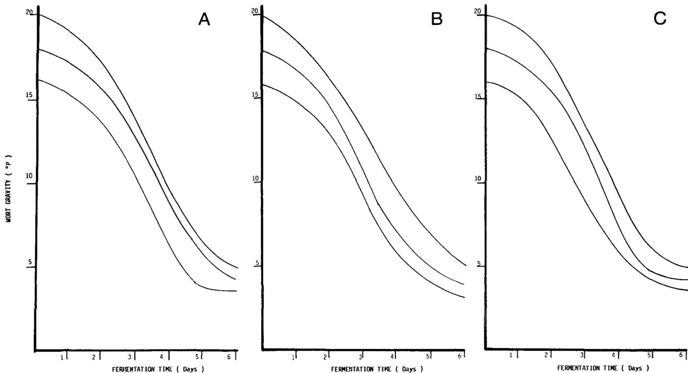
Fig. 5. Attenuation curves of high-gravity worts by *Saccharomyces uvarum* J-2036 at maximum temperatures of A, 16°C; B, 18°C; C, 20°C.
