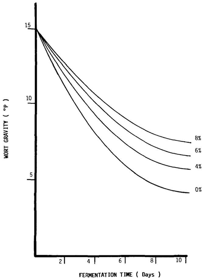
Fig. 3. Effect of ethanol concentration on the fermentative capacity of *Saccharomyces uvarum* J-3015.
