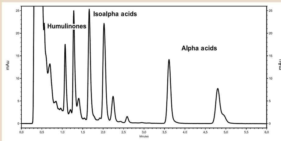
Fig. 2 HPLC trace of a commercial IPA
