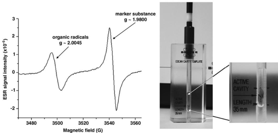
**Fig. 3.** Electron spin resonance (ESR) spectroscopy for solids. Left, Spectrum showing sample and marker signals. Right, ESR cavity where the marker substance is measured simultaneously with the solid sample (malt or barley kernel, husk, or spent grain).
