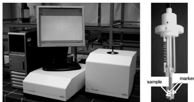
Fig. 2. Left, Electron spin resonance (ESR) spectrometer with cavity (e-scan, Bruker BioSpin). Right, ESR sample holder where marker substance is measured simultaneously with solid sample (malt or barley kernel, husk, or spent grain).
