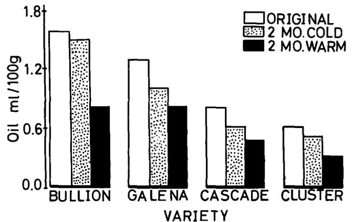
Fig. 4. Effects of room temperature and refrigerated storage on oil yields of hop samples.
