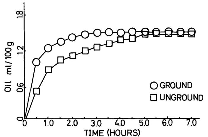
Fig. 3. Distillation rates of 100 g of ground and unground hop samples in 3 L of water. Each data point is an average of three points.
