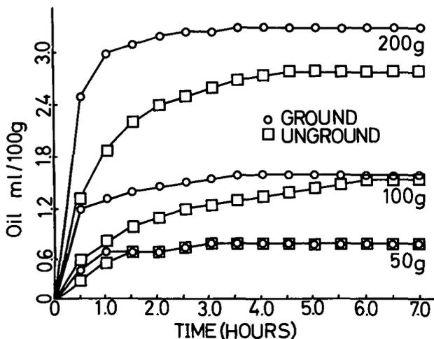
Fig. 2. Distillation rates of 50, 100, and 200 g of ground and unground hop samples in 3 L of water.
