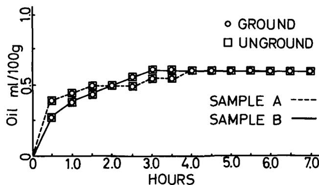
Fig. 1. Distillation rates of ground and unground lupulin.
