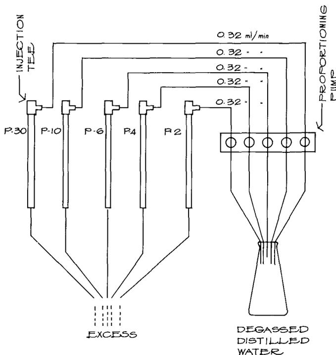
Fig. 2. Multicolumn chromatography flow scheme.
