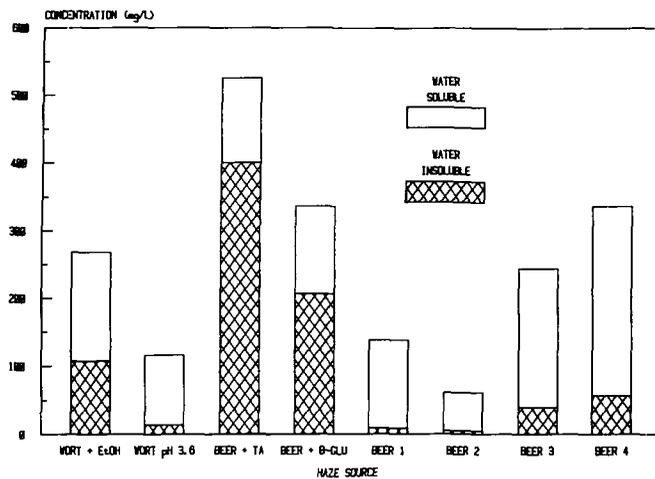
Fig. 9. Comparison of water-soluble and water-insoluble content of haze samples. EtOH = ethanol, TA = tannic acid, B-GLU =  $\beta$ -glucan.
