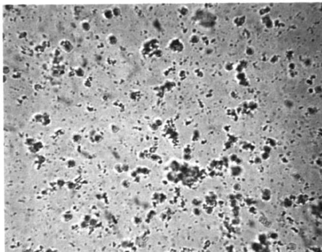
Fig. 7. Photomicrograph of haze from wort plus ethanol. Same sample and field of view as in Fig. 6 with light intensity reduced and focus shifted.
