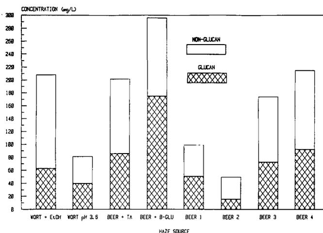
Fig. 12. Comparison of glucan and nonglucan content of haze carbohydrate. EtOH = ethanol, TA = tannic acid, B-GLU =  $\beta$ -glucan.
