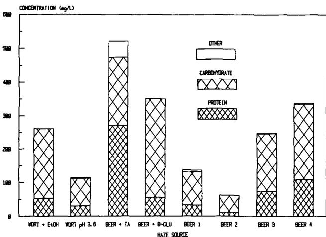
Fig. 10. Comparison of protein and carbohydrate content of haze samples. EtOH = ethanol, TA = tannic acid, B-GLU =  $\beta$ -glucan.
