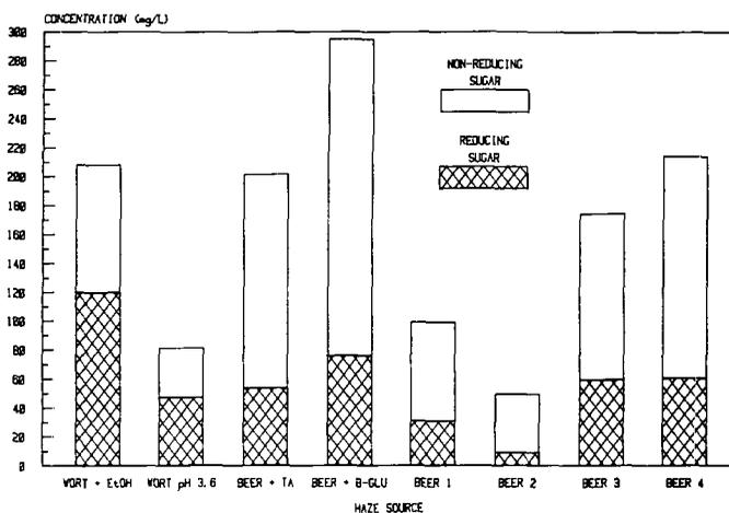
Fig. 11. Comparison of reducing and nonreducing sugar content of haze samples. EtOH = ethanol, TA = tannic acid, B-GLU =  $\beta$ -glucan.
