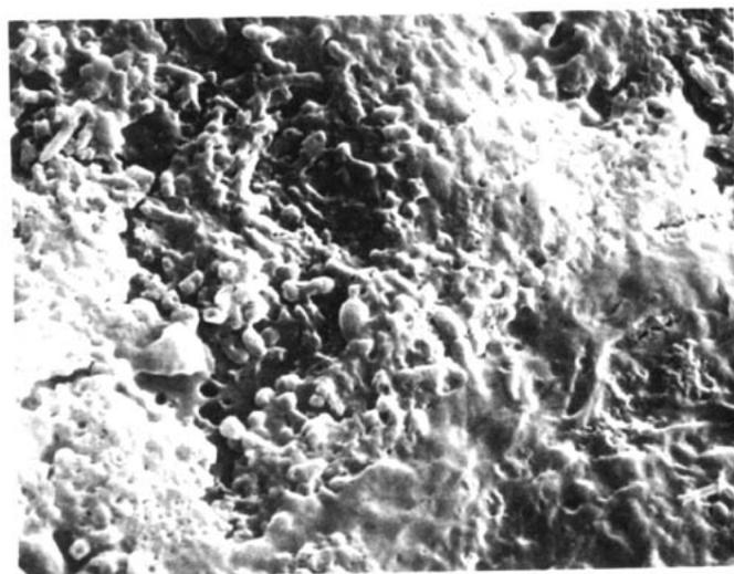
Fig. 8. Scanning electron micrograph of a haze similar to Process Beer 4 at  $\times 5,000$  magnification.
