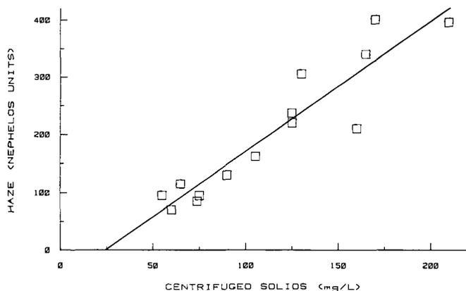
Fig. 1. Comparison of the weight of material collected by centrifugation at 13,200 × g and 0° C with the results of nephelometric measurement. All samples were drawn just before final filtration.
