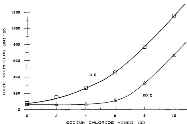
Fig. 2. Effect on light scattering of NaCl addition to beer at 0 and 20° C.
