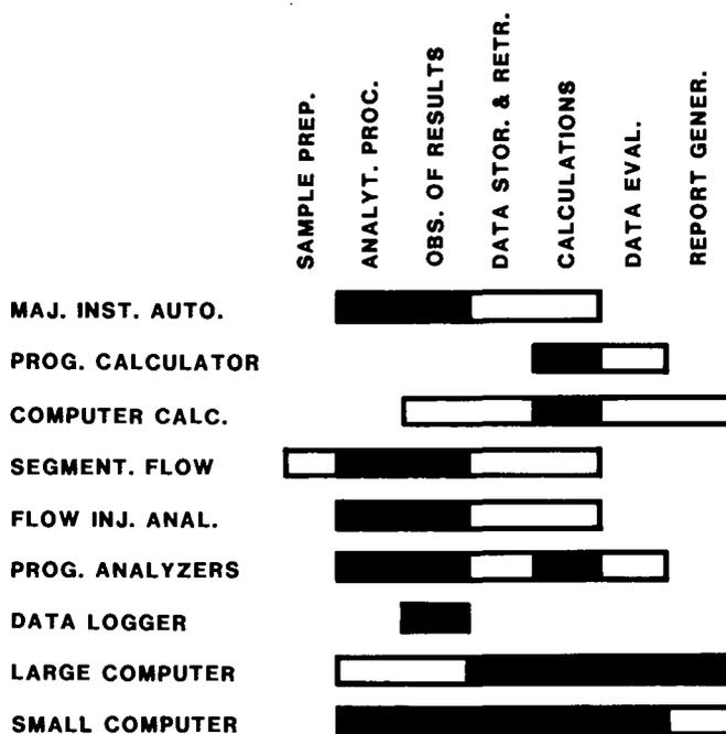
Fig. 4. Methods of laboratory automation, showing the parts of an analysis normally (solid bars) and sometimes (open bars) automated by a particular method.
