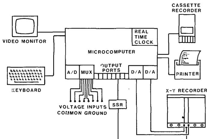
Fig. 2. Data acquisition system using a general-purpose microcomputer. MUX = multiplexer, A/D = analog-to-digital converter, D/A = digital-to-analog converter; SSR = solid state relay.
