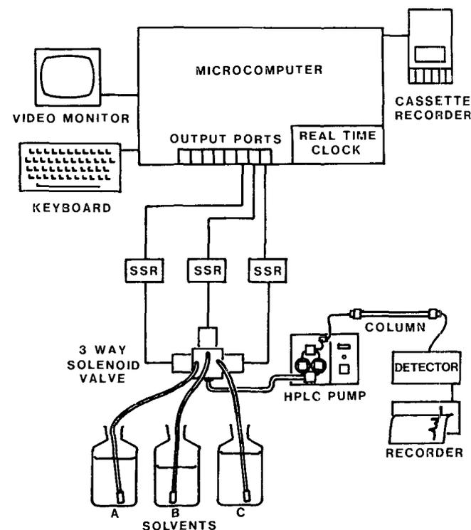
Fig. 1. A microcomputer used as a solvent gradient programmer for high performance liquid chromatography. SSR = solid state relay.
