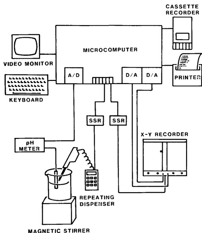
Fig. 3. A titration system operated by a microcomputer. A/D = analog-to-digital converter, D/A = digital-to-analog converter, SSR = solid state relay.
