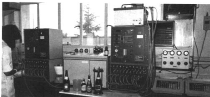
Fig. 1. The two Tekmar LSC-2 purge-and-trap systems connected to the Hewlett-Packard 5880 gas chromatograph.
