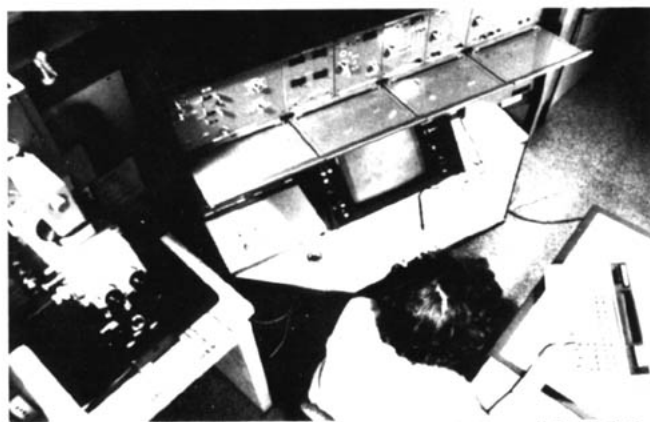
Fig. 8. Image analysis of cell wall breakdown. Left to right: Reichert Univar microscope, Quantimet 720 image analyzer, Hewlett Packard 9825 calculator.
