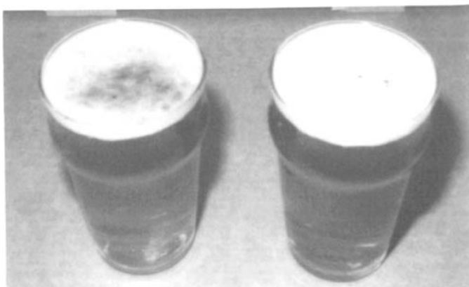
Fig. 2 The improvement in head of a lager beer from the addition of unhydrolyzed albumen. Control beer, left, beer with albumen (0.1 mg/ml), right. The beer was of OG 9°P.
