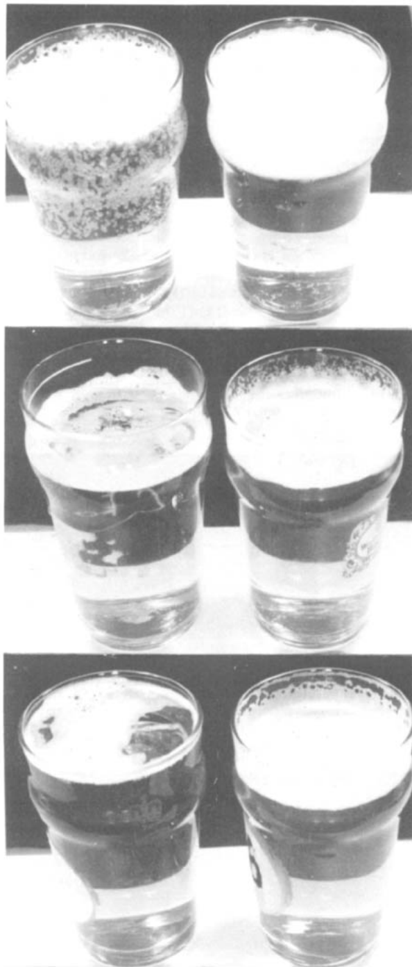
Fig. 4. The effect of ovalbumin (top), conalbumin (middle), and lysozyme (bottom) on beer foam. Control beers containing no added protein are shown on the left. Proteins were added at 0.1 mg/ml to a lager beer (OG 7.5°P).
