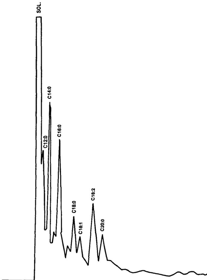
Fig. 6. Gas chromatogram of fatty acids extracted from trub.
