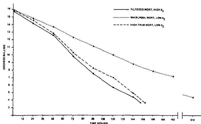
Fig. 4. Attenuation profiles for Phase 2 fermentations.
